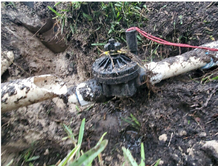
Mainline leak along Pleasant Plans was most likely the result of something driving over the valve box, pressing down on the box and snapping the pipe.
