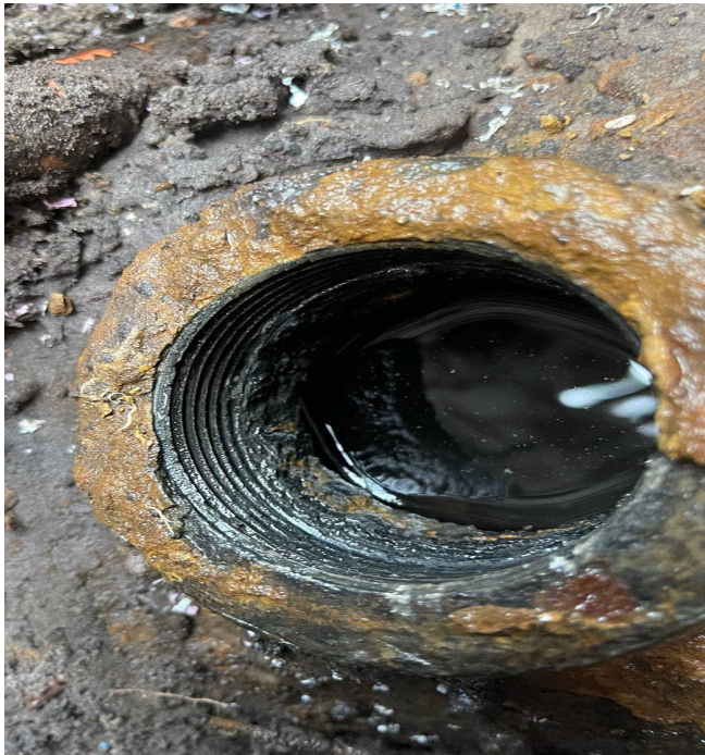
Mainline tap for valves D64 and D65. Leak was caused by a crack in the male adapter that was threaded into fitting.
